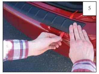
Hold the part at an angle to prevent tape from prematurely sticking and align the part on bumper by aligning shorter center rib in part with center of striker latch location and using the masking tape applied in Step 2 as a guide. Stick peeled end to Bumper and pull tab nearest the rear of the vehicle while applying downward/forward pressure to the rear edge of part.
