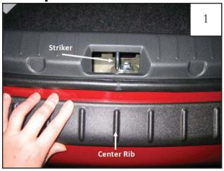
Open rear door of vehicle. WITHOUT peeling liner from tape pads, align part on bumper, the shorter center rib of the bumper protector lining up with the center of the striker latch location.
