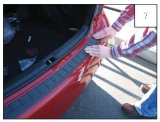
Press the part into place starting at the left side, pushing downward and forward while working your way to the right. Apply 30 PSI to the taped areas for proper bond. Tape reaches maximum adhesive bond after 24 hours of contact.
