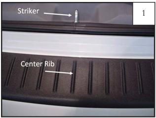
Open rear door of vehicle. WITHOUT peeling liner from tape pads, align part on bumper, centering the center rib of the bumper protector with metal loop on striker.
