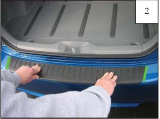
Apply a piece of masking tape along both edges of part for ease of placement during installation.
