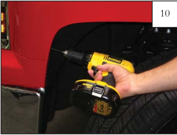
Using a 3/32" drill bit, drill pilot holes at the marks made in Step 9.
