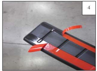
Peel red liners partially from tape pads and fold towards the outside of part.
