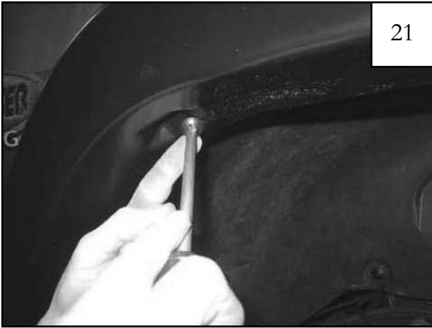
Install supplied Truss Head Screws (SW1-0057) through holes in wheel well and into #14 U-Clips installed in Step 15 (5 places).
