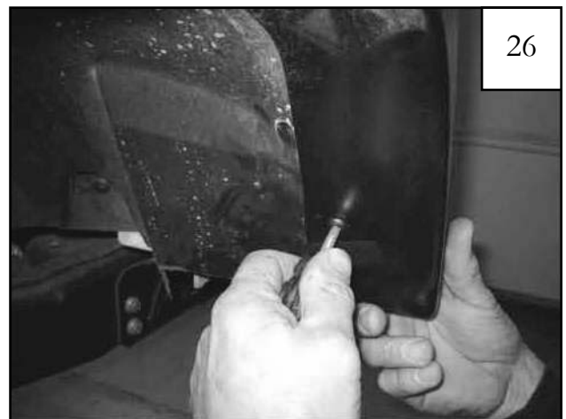
Replace splash shield, and install a supplied Truss Head Screw (SW1-0057) through rearmost hole in flare and into clip installed in Step 25. Reinstall three pocket screws removed in Step 24.
