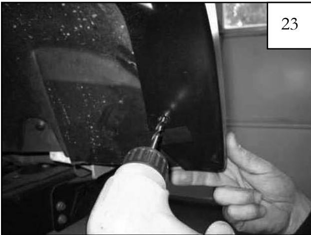
Holding the splash shield firmly, drill through rearmost hole in flare and through the splash shield using a 5/16" bit.
