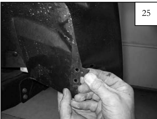
Pull the splash shield out from behind flare and install a supplied #14 U-Clip over hole drilled in Step 23. This hole will be located slightly above existing hole in splash shield.
