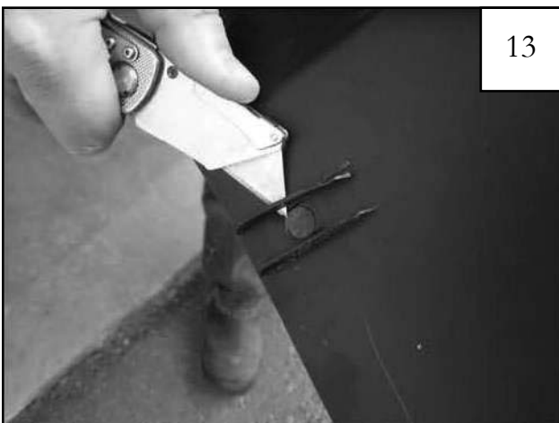
On backside of splash shield, use a utility knife to trim two plastic ribs flush with splash shield surface.
