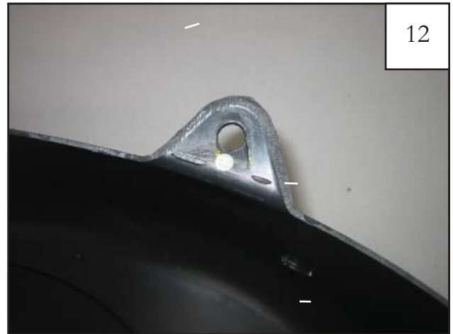
Place a grease pencil mark 1/8" below the hole on the rear mounting tab.
