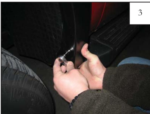
Position flare on fender, and reinstall four factory screws removed in Step 1.
