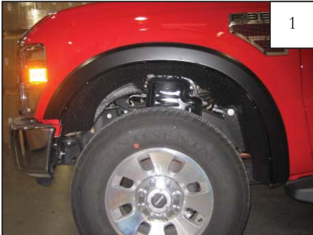
Using a 7/32" socket, remove four factory screws. Retain screws for later use.
