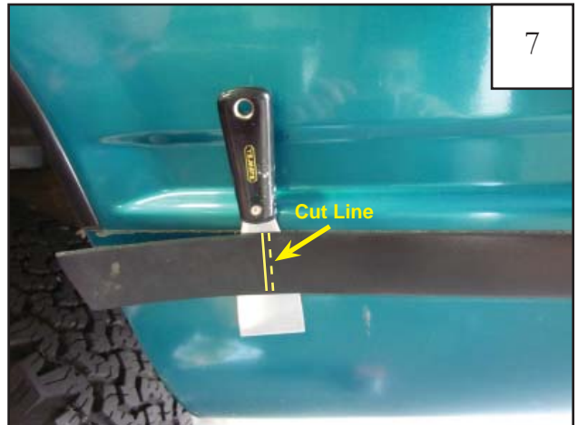
7 Slide putty knife between the molding and the body of the vehicle.
