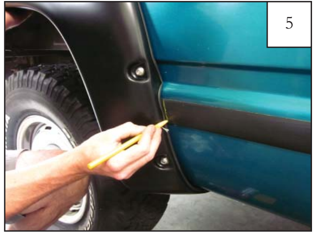
5 The factory installed body side molding (when present) will need to be trimmed to allow the flare to lay flush against the sheet metal. Hold the flare up to the wheel well opening and mark a line on the body side molding where the flare overlaps it.
