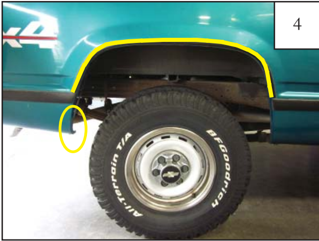
4 Remove factory fender trim and mud flaps (when installed).
