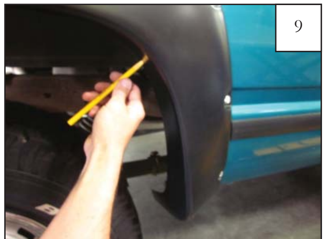
9 Hold flare in position on fender using moderate pressure. Using a grease pencil, mark five hole locations using the holes in the flare as a guide. (See Step 10)
