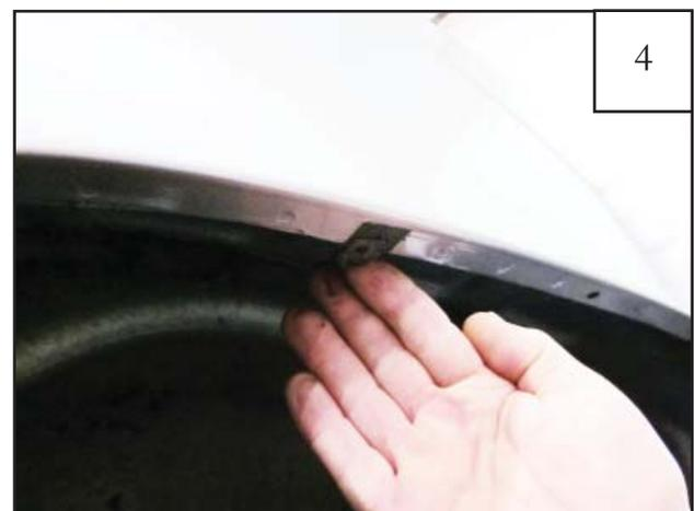
Center a supplied Clip (CL1-0022) over the upper two factory holes. *Note: The raised collar on the Clip should face upward into the interior of the fender.* Use a scratch awl to poke a hole through Tabs and factory holes.
