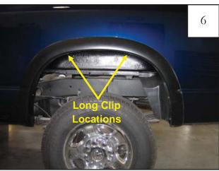
Long Clip locations. Note: Clips will be offset of fender to allow for screw to tighten.
