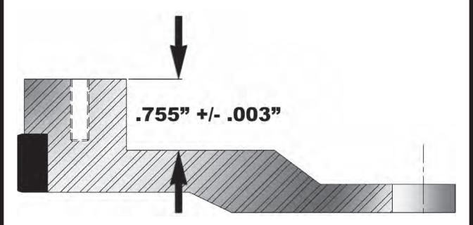
It is important to maintain the proper flywheel step specification. Failure to maintain the proper step specification may result in poor clutch performance, slipage, and/or improper release.
