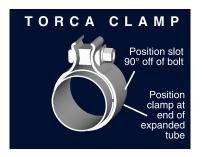
All TORCA clamps should be tightened using a properly calibrated Torque Wrench. Using an air impact gun will damage the clamp and reduce its ability to effectively seal the joint. It may also cause the joint to separate thereby causing damage to your exhaust system and your vehicle.
