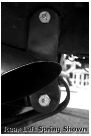
7. Once both shackles have been installed remove the jack stands from the frame and lower the vehicle to the ground. Jounce the front and rear of the vehicle to ensure it is at ride height. Torque greasable bolts to 30 ft. lbs. and non-greaseable bolts to 55 ft. lbs. Reinstall the shocks if they have been disconnected during installation and torque to spec.
