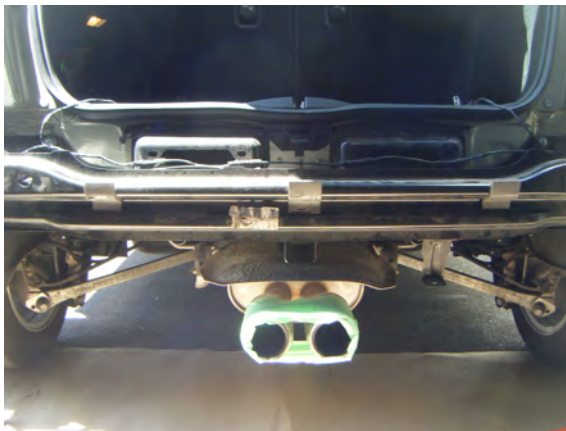
Photo 9: Hitch and bumper beam installed
