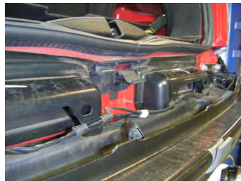
Photo 12: Center alignment feature.
