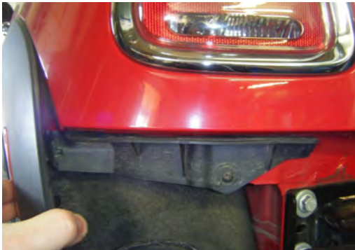
Photo 11: Side alignment feature.
