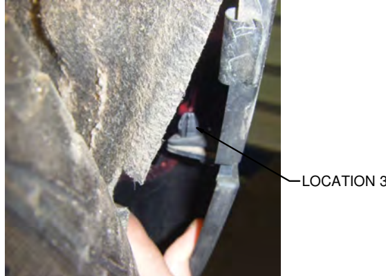
Photo 3: Fastener B behind rear wheel well liner.
