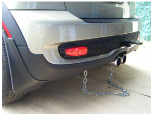
Photo 13: Hitch shown installed with safety chains
