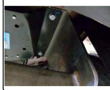
5. Trim heat shield as shown and install heat shield using two (2) hex nuts removed in step 1 and discard the other two (2) hex nuts. Raise exhaust back into position by reattaching rubber exhaust hangers to hanger rods.
