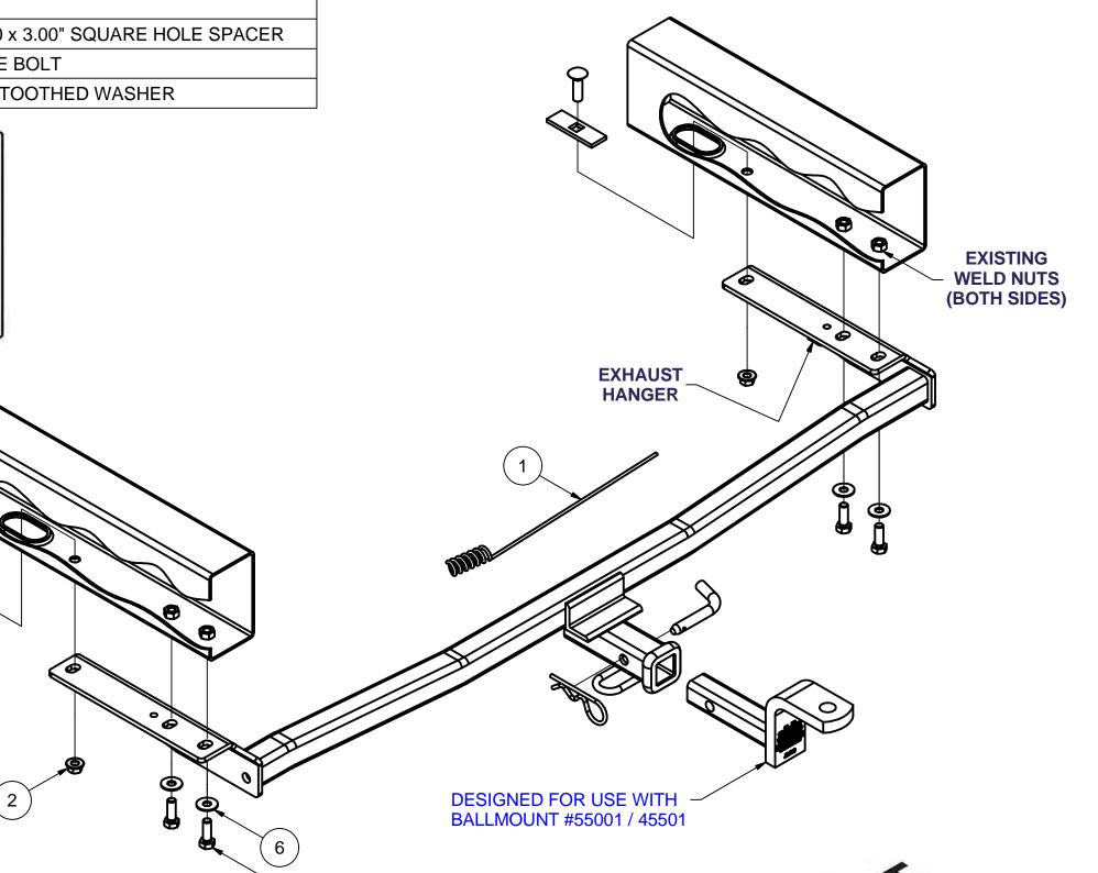
HITCH WEIGHT: 25 LBS. INSTALL TIME PROFESSIONAL: 30 MINUTES NOVICE (DIY): 60 MINUTES INSTALL NOTES: - NO DRILLING REQUIRED
