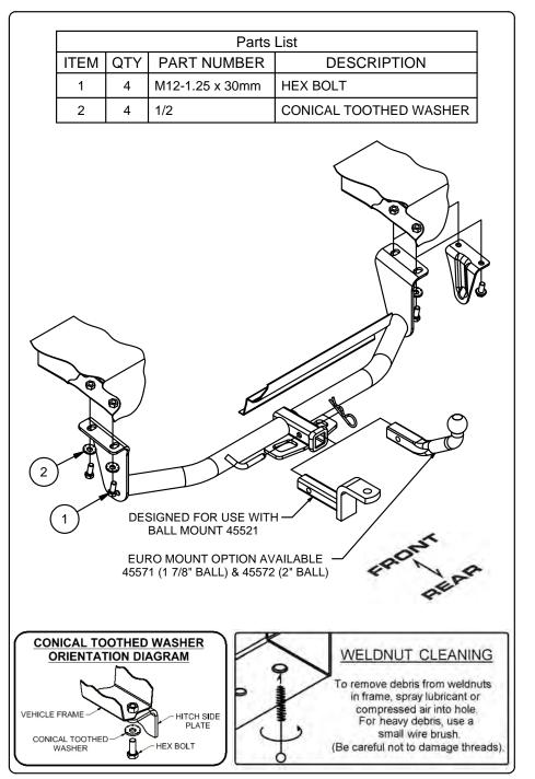
1. If present, remove existing bolts from tow loop(s). Return tow loop(s) and bolts to owner.
