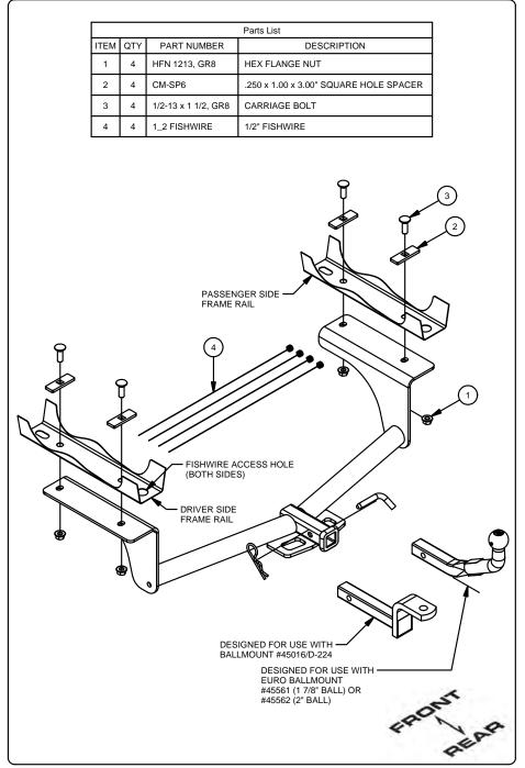
1) Fishwire the four (4) 1/2-13 carriage bolts and the CM-SP6 spacers into the vehicle frame through the access holes as shown. Refer to the "Fishwire Technique" diagram.
