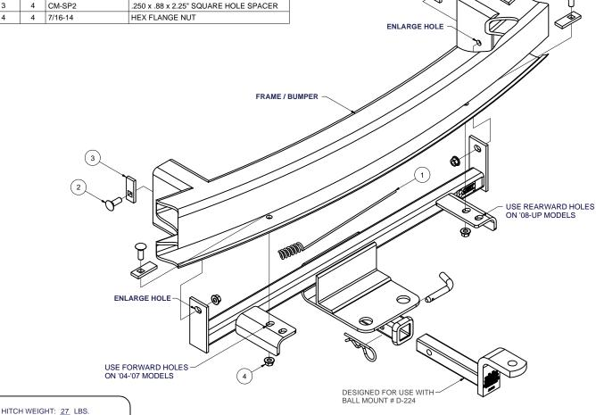
HITCH WEIGHT: <u>27</u> LBS. INSTALL TIME: <u>25</u> MINUTES INSTALL NOTES: - ENLARGE HOLES
