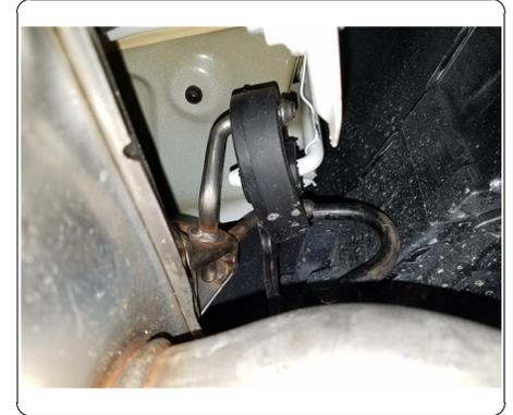
2. Locate and remove (3) bolts with a 10mm socket to remove the heat shield. Mark out a 9.25" x 10.50" section using masking tape and trim the heat shield. Reinstall heatshield. **NOTE:** If vehicle is dual exhaust remove (6) bolts and trim (2) heat shields. Reinstall after trim.
