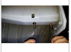
Raise hitch into position running the fishwires through the holes on the hitch. Remove fishwires and loosely fasten (4) 7/16" flange nuts.
