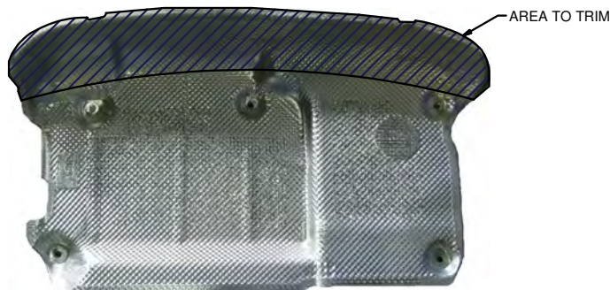
HEAT SHIELD TRIMMING DIAGRAM
