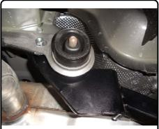
Raise the center section of the hitch into place and secure the (5) 1/2" hardware that hold it into place. Torque 1/2" hardware to 75 lb-ft. Installation is complete.
