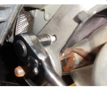
2. Raise receiver tube section of hitch into place and use the 8mm bolts and conical toothed washers provided and secure into place.
