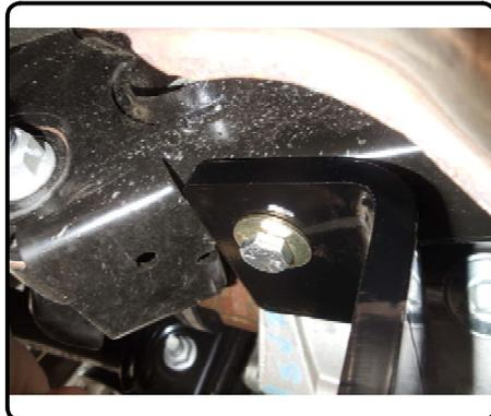
6. Raise the center section of the hitch into place and secure the (5) 1/2" hardware that hold it into place. Torque 1/2" hardware to 75 lb-ft. Installation is complete.
