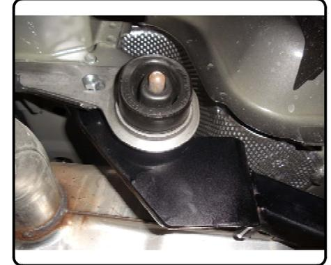
4. Assemble the bolt on bracket as shown. Tighten 3/8" bolt to 30 lb-ft.
