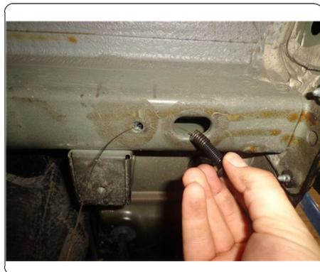
5. Reverse fishwire 1/2" carriage bolts and SP10 spacers through the access hole. Carefully pull bumper cover and raise hitch into position. Loosely fasten the hitch using 1/2" flange nuts on both sides.
