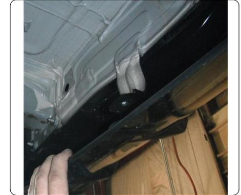
2. Remove (2) M8 fasteners for the driver side exhaust bracket, and (2) M8 fasteners for the muffler hangers using a 13mm socket. Support the muffler to prevent damage to the exhaust.
