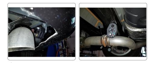
Locate and remove (2) plastic nuts with a 10mm socket. Remove heat shield and mark out a 5" x 13" section with masking tape. Use aviation shears to trim marked area. Reinstall with (1) nut using a 10mm socket.
