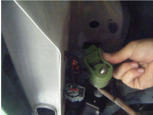
EXHAUST HANGER REMOVAL
