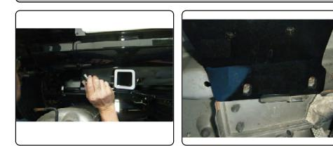
4. Secure the passenger side using the existing weld nuts, the M12 hex head bolts and the 1/2" conical toothed washers provided.
