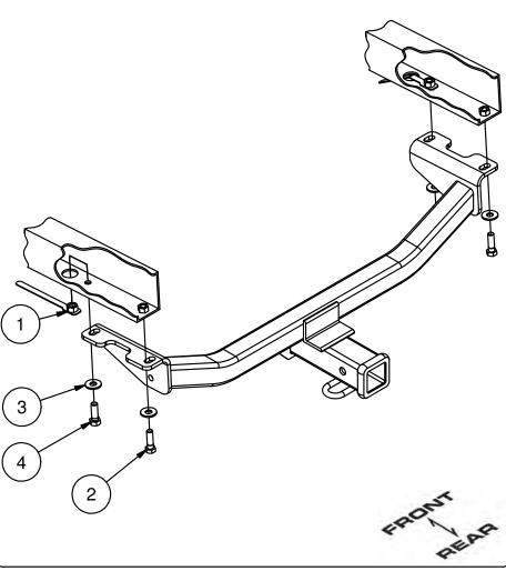
1. Locate (2) existing weldnuts in rear of vehicle frame. Spray lubricant or compressed air into hole. For heavy debris, use a small wire brush. (Be careful not to damage threads.)
