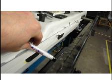
6.) Remove bumper beam using a 16mm socket (2 bolts each side) and a 15mm socket (1 nut each side).
