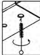
To remove debris from weldnuts in frame, spray lubricant or compressed air into hole. For heavy debris, use a small wire brush. (Be careful not to damage threads).
