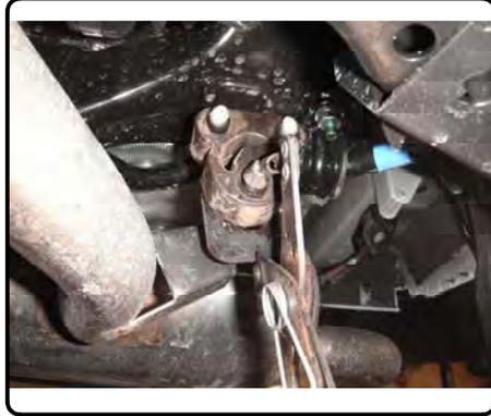
4) Raise hitch into position and secure with hex bolts and conical washers as shown in the diagram above.
