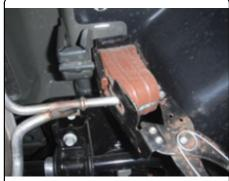
2) Using a die grinder, enlarge the forward most hole on the side of both frames to accept the supplied spacers and carriage bolts. Fishwire (2) CM-SP4 spacers and (2) 1/2" carriage bolts into the mounting holes as shown for both frames.
