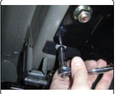
6) Raise the exhaust back into position and reinstall rubber isolators.
