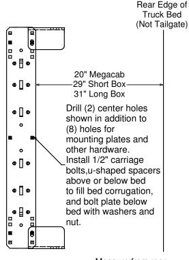
Measure from rear edge of truck bed to rear edge of mounting rail
