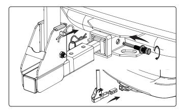
**Note:** To adapt the 1 1/4" shank to fit a 2" receiver tube opening, assemble the U-type adapter (#4) onto the 1 1/4" shank (#3). Align the holes and secure with 1/2" hex head bolt, flat washer, star washer and clip (#9).
