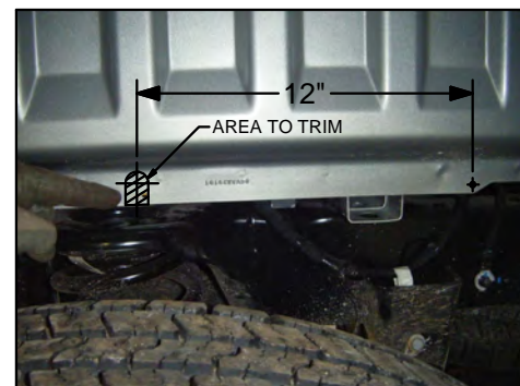
Figure 10.1: Inside Driver Side Rear Wheel Well
