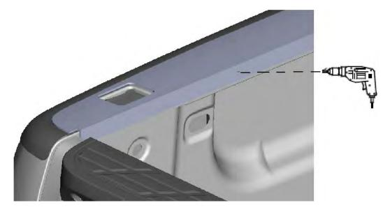
Secure the bed cap to the vehicle bed rail using a 1/4" x 1" ribneck carriage bolt (C), a 1/4" flat washer (D), and a 1/4" hex nut (E) at the mounting locations drilled into the bed rail.
