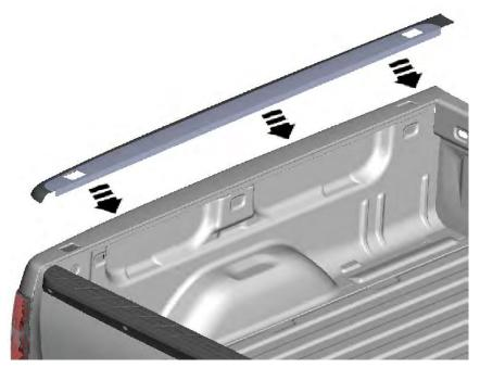
Once everything is lined up, firmly press down on the top and sides of the bed cap for 30 seconds to ensure that the bed cap properly adheres to the vehicle.
