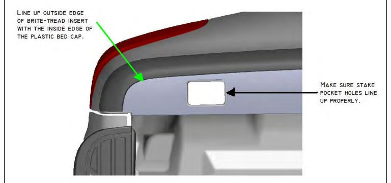
Note: There may be a gap between the plastic bed cap and the brite-tread insert where the two profiles meet. This gap will be taken care of in step 4.
