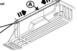
If plastic spacers (F) have been provided with your side bedcap, then place them at the front and rear of the vehicle bed rail between the inside edge of the side bedcap (A) and the vehicle bed rail as shown below.
