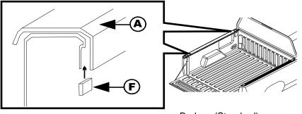
Apply pressure to the side bedcap (A) as shown below to adhere the tape on the side bedcap (A) to the vehicle bed rail.
