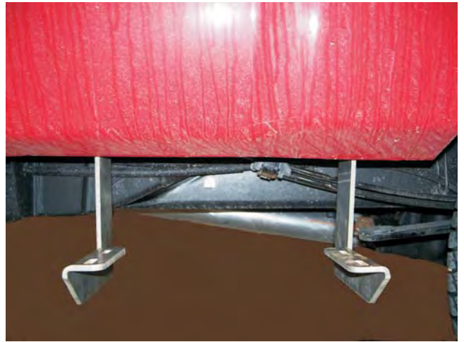
Bent flange on Braces should face each other.
