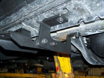
Place running board (A) onto the brackets. Align 8mm square head bolts (H) in the bottom of the running board (A) with holes in the brackets. Completely tighten brackets to vehicle. Center board on vehicle between wheel well openings or until desired appearance is aquired. Adjust board in/out on vehicle until desired appearance is met. Secure board into palce using 8mm hex nuts (L).
