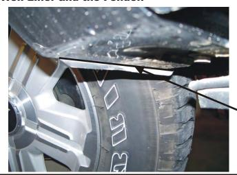
The Wheel Well Liner does not need to be cut in Option #2
