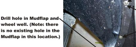
**►**Use holes in Mudflap as a guide for drilling holes.
