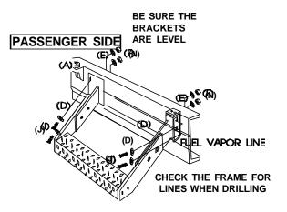
(#3) After marking the frame, move the step assembly out of the way and drill 3/8" holes at each of the marks on the frame.
