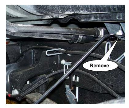
Attach the driver side-cross brace (F) to the bottom side of the wheel well stiffener with the bolt removed in the previous step.
