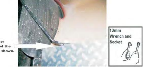
Make sure stiffener is resting on top of the running board as shown.
