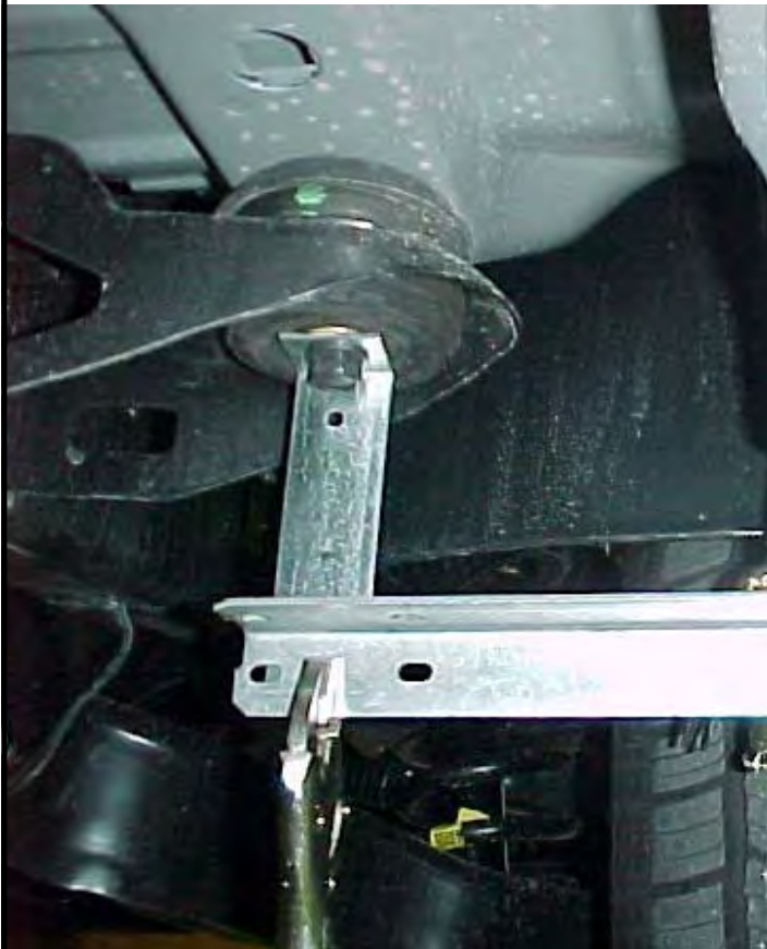
Front Body mount - Clamped into position
