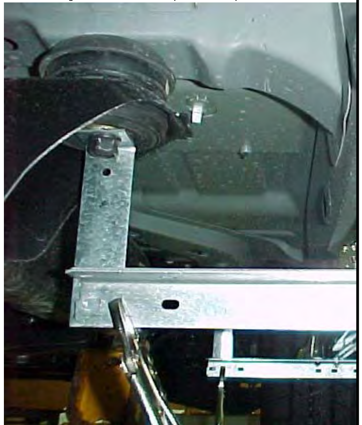
Rear Body Mount - Clamped into position
