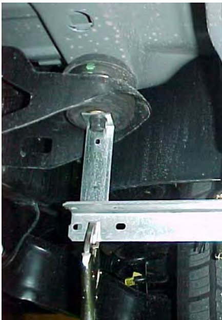
Front Body mount - Clamped into position
