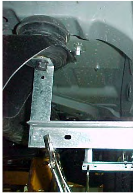
Middle Body Mount - Clamped into position
