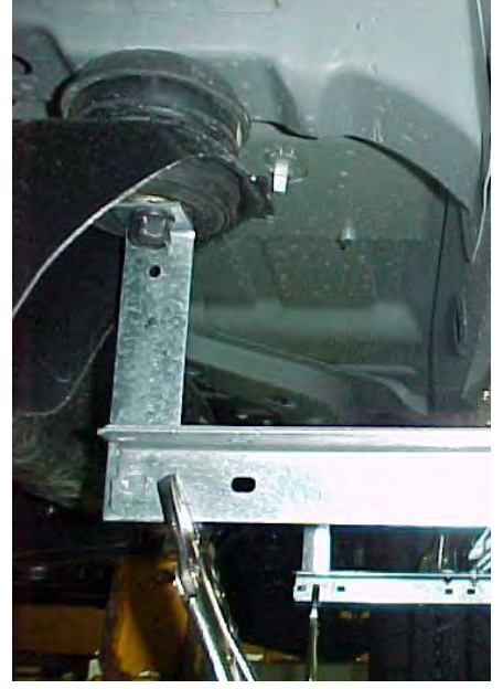
Rear Body Mount - Clamped into position
