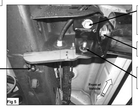
12mm x 120mm Hex **Head Bolt** 12mm Lock Washer 12mm Flat Washer NOTE: For 06-On vehicles use factory bolt.
