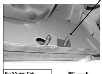
Fig 5 Super Cab passenger side rear mounting location pictured. Shown with Plastic Retainer in place
