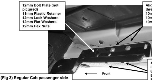
Align holes in brackets with threaded holes in 10mm Clip Nuts. 10mm x 30mm Hex Bolts 10mm Lock Washers 10mm Flat Washers
