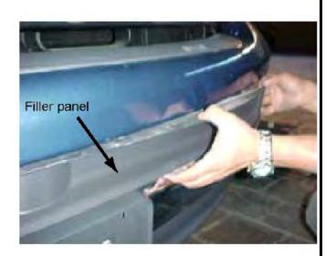
3 - Use the enclosed templates as a guide to trim out the bumper fascia that was removed in step 2 of this instruction. Place the template onto the outer edge of the bumper fascia (filler panel) and then trim out around the template. Repeat this for the opposite side of the bumper fascia. Replace the bumper fascia and the plastic rivets on the vehicle.
