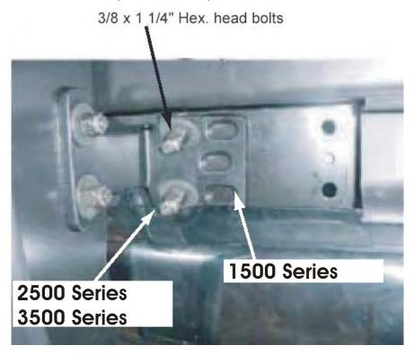
5 - Open the hood on the vehicle and locate the existing 8mm bolt on the frame cross member. Remove the existing 8mm bolt from the vehicle and attach the auxiliary mounting bracket to this location as shown below using the enclosed 8mm x 25mm hex head bolts, 3/8" lock washers, and 3/8" flat washers.
