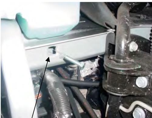
Here, insert the M10 bolt with guide
